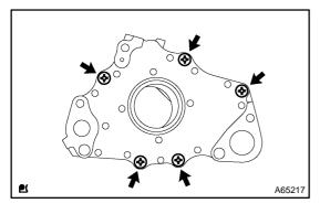
(h) Install the oil pump cover with 5 screws.
