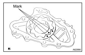
(g) Install the oil pump rotor.
