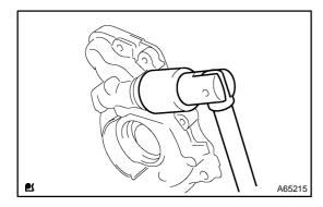
(b) Using a 28 mm socket wrench, install the oil pump relief valve plug.
