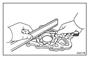
(f) Check the rotor side clearance.
